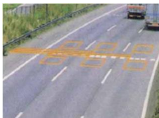
Vehicle Detector (Inductive Loop Detector)
